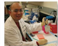
Figure 6.7. A multichannel pipet speeds setting up the reaction because it allows for pipetting several samples at the same time. Photo courtesy of Cell Genesys, Inc.
