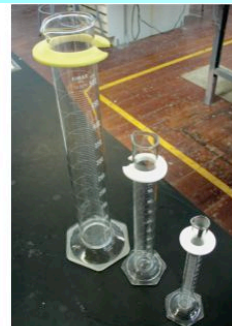
Figure 3.2. Graduated cylinders are used to measure volumes between 10 mL and 2 L. Photo by author.
