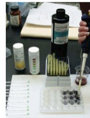
Figure 6.5. Prepare everything before beginning. Be careful to not cross contaminate samples. Change tips with each measurement. Photo by author.
